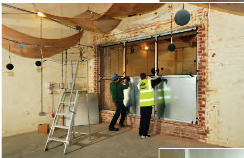
Fitting Frame and Panels into Test Aperture
