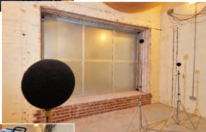
Microphone Positions in Receiving Room
