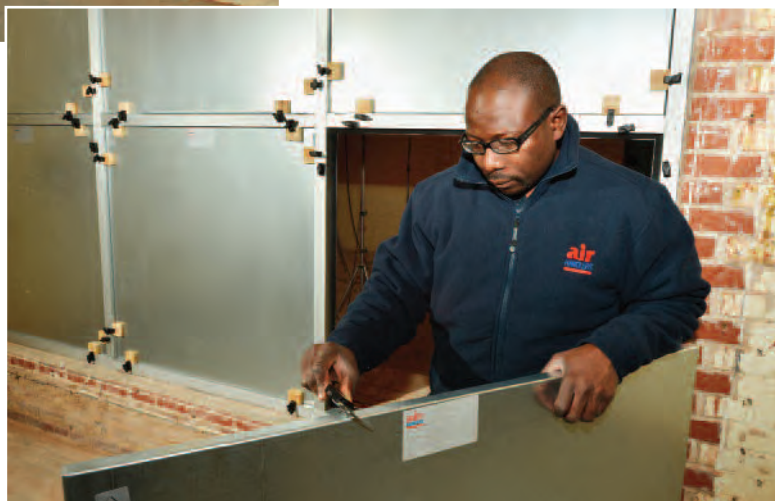
Fitting Frame and Panels into Test Aperture
