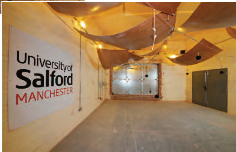
Plywood Diffusers Receiving Room
